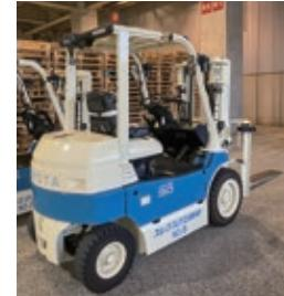
Electric forklift equipped with a lithium-ion battery
